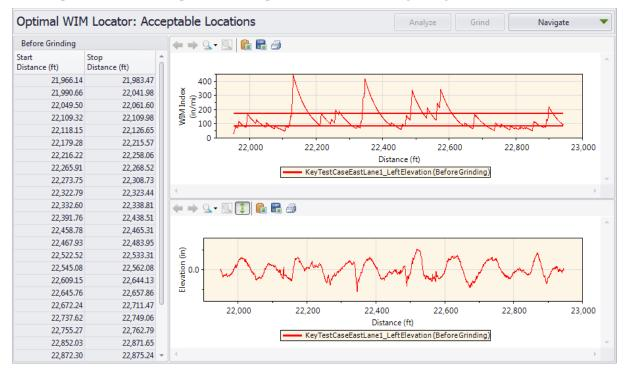
An example of a WIM index report with a comparison chart and (auto-grind) grinding results: This is a powerful combination of charts to examine grinding effects on the WIM index report. Therefore, an adequate grinding strategy can be selected to obtain a desired location for a WIM site.
