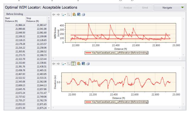
An example of WIM index report with a comparison chart and (auto-grind) grinding results: This is a powerful combination of charts to examine grinding effects on the WIM index report. Therefore, an adequate grinding strategy can be selected to obtain a desired location for a WIM site.
