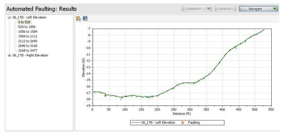
The lower chart shows the location and height of each fault.
