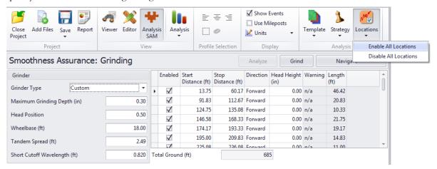
Spot grinding locations can be displayed as orange-coded segments on the map. Mouse over each grinding spot to show information include the start and stop distances.
