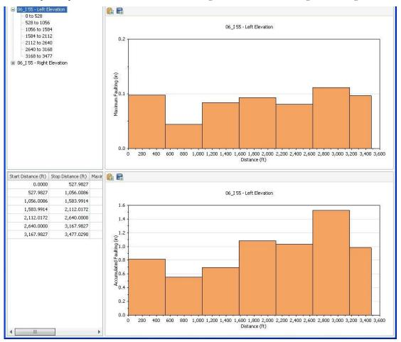
Use the Navigate button to switch to the Joint Locations view. The top chart shows joint spacing in comparison to the nominal joint spacing specified in the inputs.
