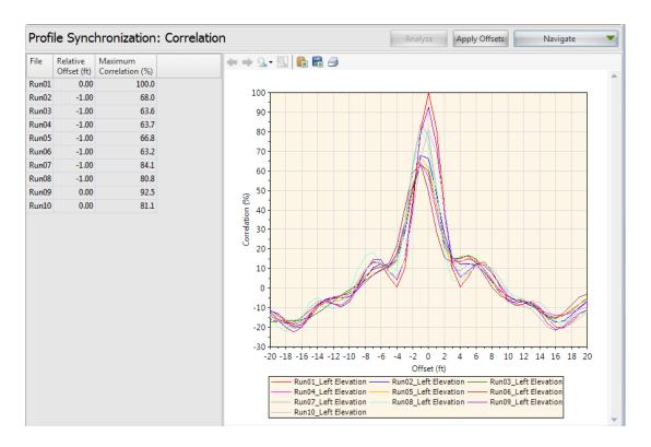
▶ Shifted Profiles Chart (Elevation) - Basis profile compared with the shifted comparison profile.
