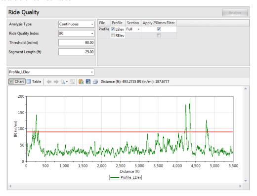
**Fixed Interval** analysis results. You can select each file to display the analysis results. Toggle between the chart, table, and map data (if a route is defined). Color-coded segments on the map indicate pass (blue) or fail (red). Mouse over each segment to show information including the start/stop distance and the ride index value.
