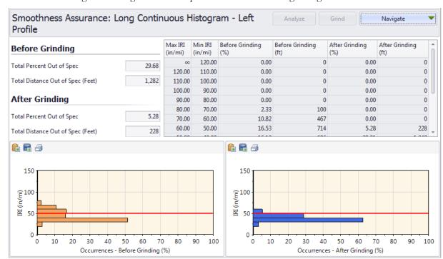
A view of the histograms of long continuous reports for before and after grinding:
