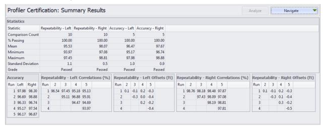
The detailed results contain additional information about each repeatability and accuracy comparison. Statistics include correlation, shape coefficient, roughness coefficient, offset, basis IRI, comparison IRI, and IRI difference.
