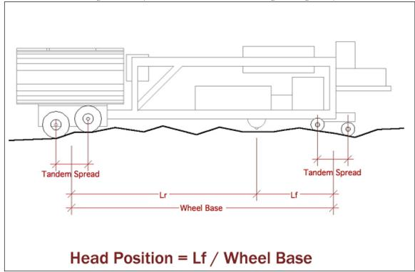
The above diagram does not include an additional support wheel to reflect grinder dimensions during grinding operation.
