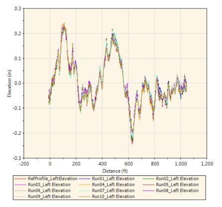
▶ Shifted Filtered Profiles Chart (Slope) - Basis profile slope compared with the shifted comparison profile slope, after filtering (if applicable).
