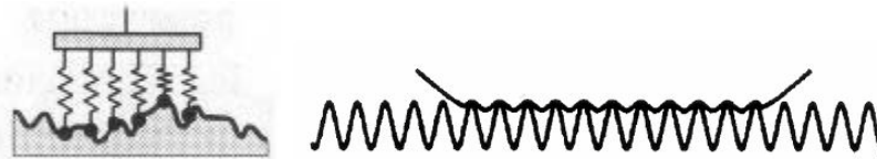
Figure 1. Fixed footprint tire model and illustration of tire-tread penetration into pavement textures. (Karamihas, 2005)
